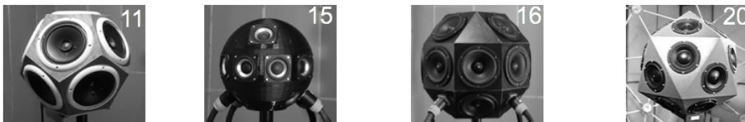
Figure 3.1: Compact spherical loudspeaker arrays at the IEM and their number of transducers. The 3|9|3 array (3 + 9 + 3 = 15 loudspeakers) is a promising prototype of a mixed-order array that needs further evaluation through listening experiments.
