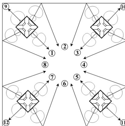
Figure 3.2: Principle of surround-with-depth using first-order cubical loudspeakers as published by Deppisch et. al. [6]. With multiple higher order beamformers (higher spatial resolution) a more enveloping sound scene might be achieved.
