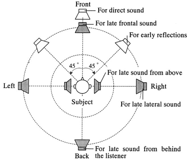
Figure 2.1: Illustration of the experimental setup to investigate the influence of late sound arrival direction on LEV (Furuya et. al. [8]).
