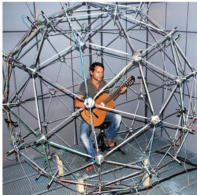
Figure 1 Large scale microphone array with 64 NTI measurement microphones. The singers are supposed to stand inside the array while getting cues from a screen and via talkback. A tracking system should measure the head movements and a video camera will be used to study the relationships with mouth opening and posture.
